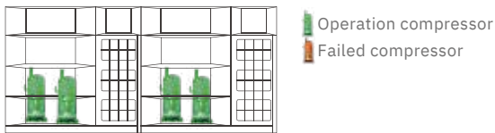
Intelligent load-bearing between units during normal operation
